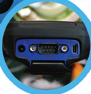
Wi-Fi, Bluetooth, GPRS modem, 5 MP camera, voice call and MMS mini waterproof USB connector, RS232 serial port
